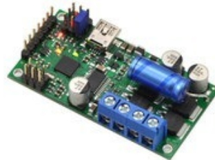
Simple High-Power Motor Controller 18v25 or 24v23 with included hardware installed.
