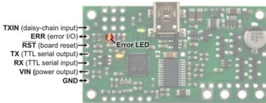
Simple Motor Controller 18v7 serial connections.
