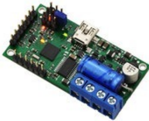
Simple Motor Controller 18v7, fully assembled.
