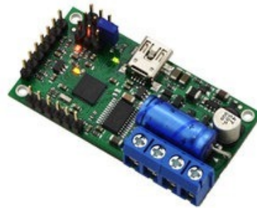
Simple Motor Controller 18v7, fully assembled.
